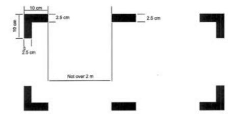
(b) If the corner markings are more than 2 m apart, intermediate lines 9 cm x 3 cm shall be inserted so that there is no more than 2 m between adjacent markings.
